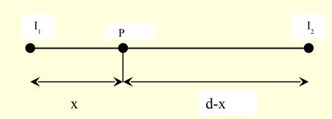
Let P be the point where the screen is placed so it will be equally illuminated by the two sources, and let x be the distance of P from  $I_1$ . Equating the two expressions for intensity of illumination, we have
